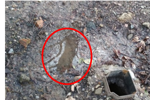
Small puddle – without remote water logger would anyone think this was above a 44,000 litre a day water leak?
